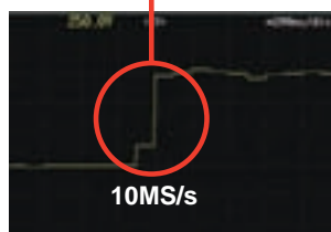
Example: Same inverter output waveform measured at 10 MS/s and 100 MS/s
