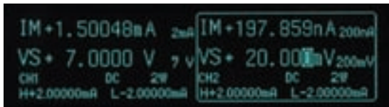
2-channel display example (256 x 64 dot matrix display)
