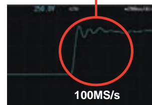
Example: Same inverter output waveform measured at 10 MS/s and 100 MS/s
